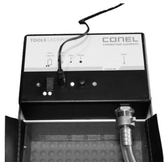
The Leak Pump is now always ready for use if there is 220V voltage at the mains plug of the power supply. If the 220V mains voltage fails, the Leak Pump continues to run on battery power. The same operational readiness information then applies to mains free battery operation. If the mains failure is over, the pump runs again via 220V mains voltage. As long as the pump is not running, the battery is recharged if necessary.
